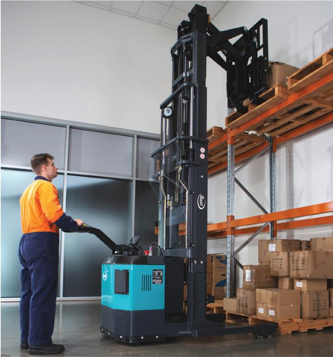
Lift loads over 5 meters high with a reach of almost 600mm
